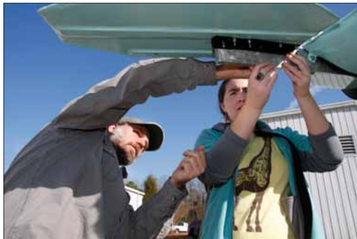
ENGINEERS WITHOUT BORDERS members Jeff Harmin, graduate student in electrical and computer engineering, and Sarah Peterson, junior in biomedical engineering, work to attach the tail to their homemade wind turbine before erecting it outside of the Applied Energy Research Lab. Photo by Tim O'Brien
